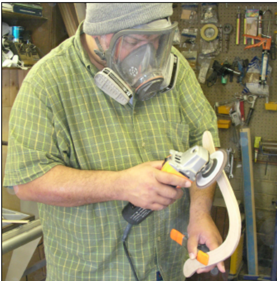
John likes the "hands-on" feeling of using a grinder while holding the blank in his hands.
