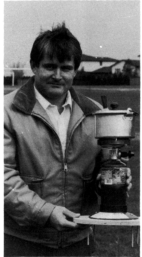
Ontario, Canada's John Cryderman shows a portable propane steam-tuning blast furnace you can build for about $50.
